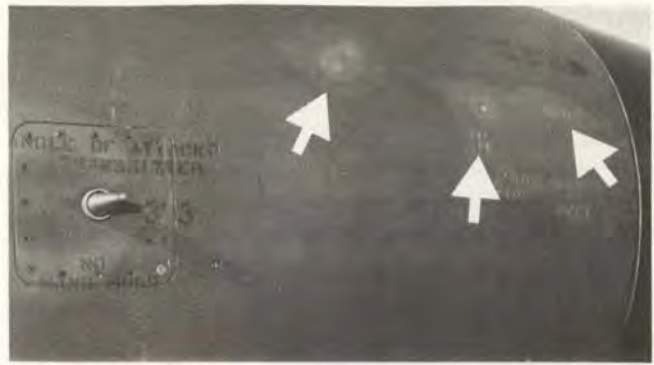
FIG. 7 Pit marks where flash attached
