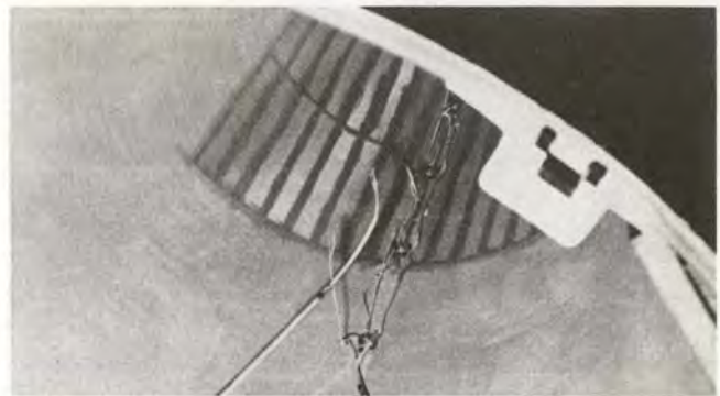
FIG. 9 Typical lightning damage to pitot static lines and heater power cord
