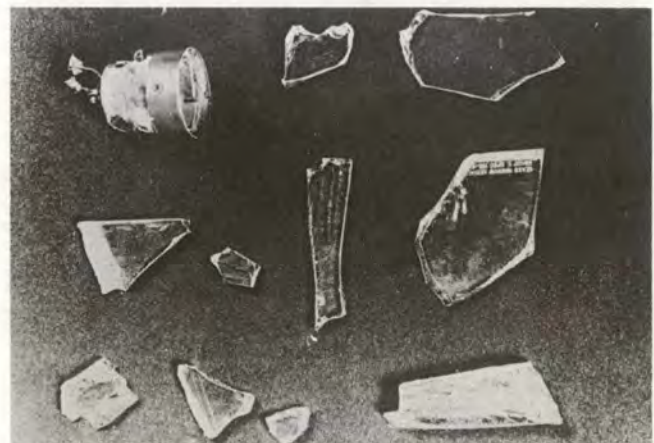
FIG. 10 NAV light globe broken by lightning, leaving a path for lightning current to enter aircraft's electric system.
