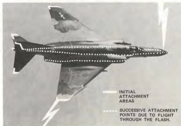
FIG. 4 Lightning Attachment Points
